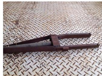
*Tool created by the producer to help clip wire into posts.*
