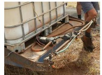
*The producer built a boomless spray to control vegetation along fence. Sprays with Roundup twice a year, depending on season.*
