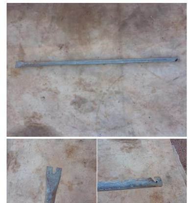
*Tool created by the producer to clip wire into posts.*
